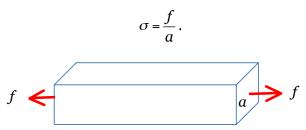
**Force per unit area. Traction.** We now generalize these familiar examples to a fluid in a general homogeneous state. Inside the fluid, consider a planar region of area a, normal to a unit vector  $\mathbf{n}$ . Acting on the planar region is a force  $\mathbf{f}$ . In general, the force has components normal and tangential to the plane. Define the traction  $\mathbf{t}$  by the force acting on the planar region divided by the area of the region:
