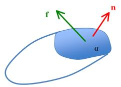
**Stress**. For a fluid in a homogeneous state, how many independent quantities do we need to specify its state of stress? The answer is six. To see this answer requires a deeper generalization than the definition of traction.
