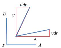
**Velocity gradient.** Consider two points P and A, of coordinates  $\mathbf{x}^P$  and  $\mathbf{x}^A$ , and velocities  $\mathbf{v}^P$  and  $\mathbf{v}^A$ . When a fluid undergoes homogeneous deformation, the velocity of material particle is linear in the position of the material particle:
