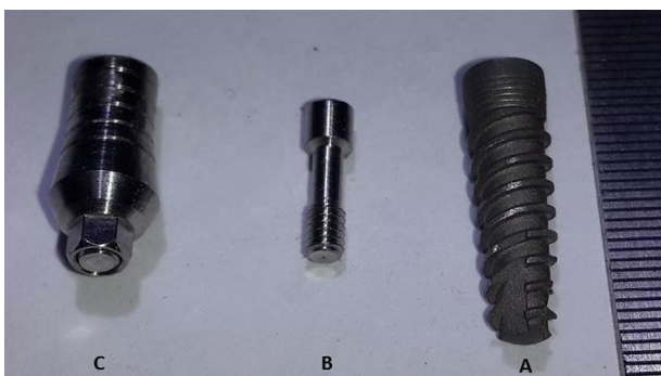
Fig. 1 – Tested implants and implant's parts. A: Implant body. B: Abutment screw. C: Implant abutment.
