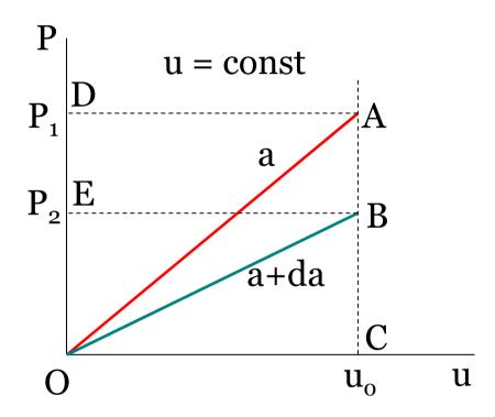
No external work done  $U_2 < U_1$  Decrease in strain energy – used for crack growth
