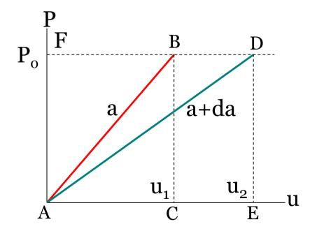
Write total potentials when crack sizes are 'a' and 'a+da'
