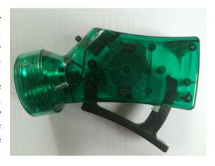
**Demonstration**. Bring a generator to class. The movement of my hand rotates a disk. The rotation induces an electric current in an electric circuit. The electric current lights up a bulb.
