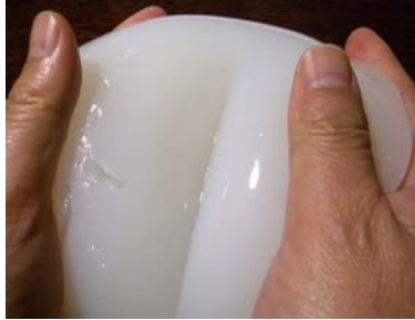
FIG. 1. A crease formed on the compressed surface of a popular Chinese food, Liang Fen (a starch gel).
