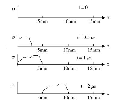
**Longitudinal wave in a rod.** The speed of sound in steel is  $\sim 5$  km/s. Imagine that a hammer hits one end of a steel rod. The hit starts at time zero, and lasts for 1  $\mu$  s. A frame-by-frame "movie" shows the stress profiles at several times.
