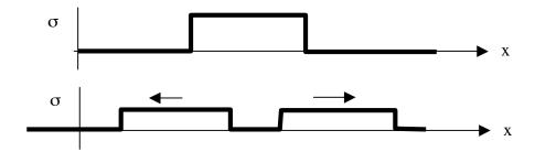
**Reflection from a free end.** We next illustrate how boundary conditions come into play. An incident wave in the rod hits the free end of the rod, and reflects back into the rod.
