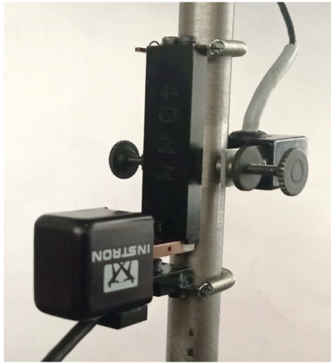
Fig. 3-4. Longitudinal and transverse extensometers on the specimen for Poisson's ratio determination.
