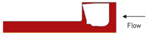
Figure 3: Axisymmetric model of the flow path
