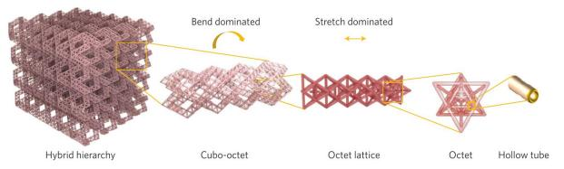
Fig.1 Example of a hierarchical lattice architecturation strategy combining bending and stretching [4]
