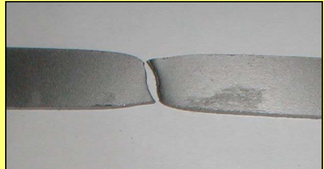
Figure 8 - Tensile specimen pulled to fracture. Depicts region where necking occurred.
