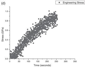
Figure 2. A typical brittle-like fracture of a long nanowire under tension with a low loading rate (~0.1nm/s): a) initial state; b) after breaking (scale bar 10nm); c) corresponding engineering stress-strain curve; d) engineering stress as a function of loading time.
