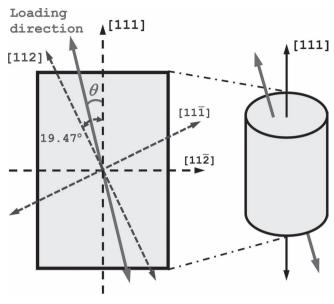
Figure 6. Schematic illustration of loading misalignment with corresponding multiple slip systems for twining partial and normal partial dislocation initiation: the bold red solid line with single-head arrow stands for the loading direction with a misalignment angle theta; and the dotted black (blue) lines with single-head arrow indicate two possible partial dislocation slip systems.
