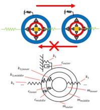
Lattice with internal nonlinear multi-scales and coupling asymmetry resulting in global non-reciprocal acoustics (top); cell model (bottom).
