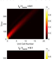
Simulations for boundary impulses: spatiotemporal cell energy evolution for left (top) and right excitation (bottom).
