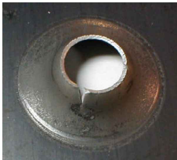
Figure 2 - Hole expansion specimen tested to failure.
