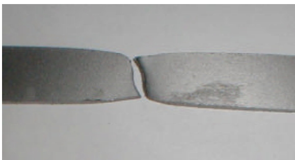
Figure 1 - Tensile specimen pulled to fracture. Depicts region where necking occurred.
