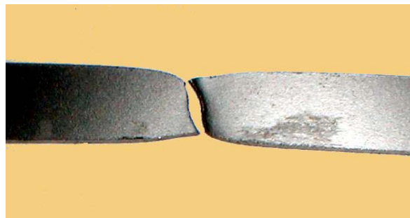
Figure 1 - Tensile specimen pulled to fracture. Depicts region where necking occurred.
