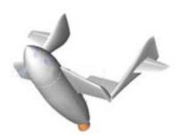
Figure 6<sup>13</sup>. Feathered configuration of SpaceShipOne during reentry.
