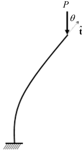
Figure A.2. Schematic of a clamped-free elastica subjected to a vertical point load.
