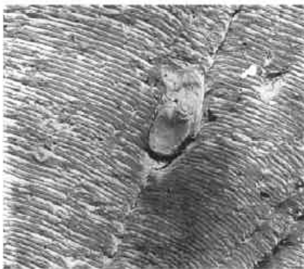
Figure 2.23 Typical striations around an inclusions [8]
